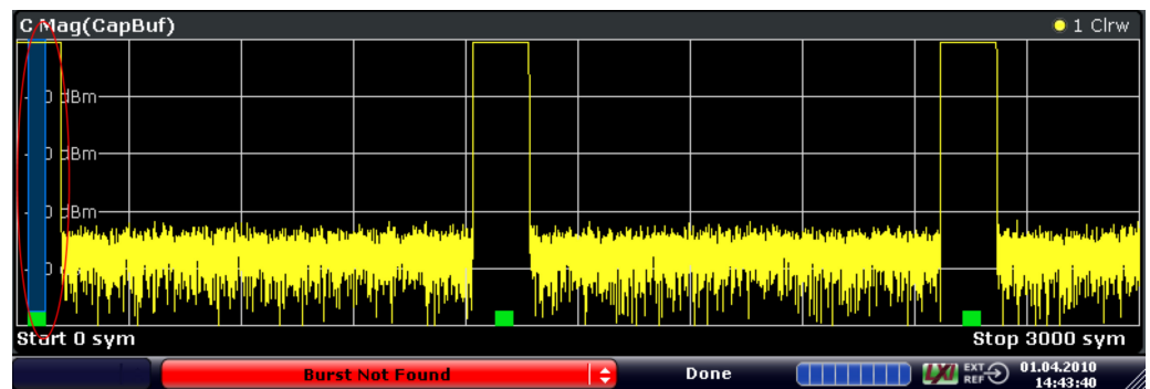
Fig. 10-3: Example for measurement on incomplete burst capture
