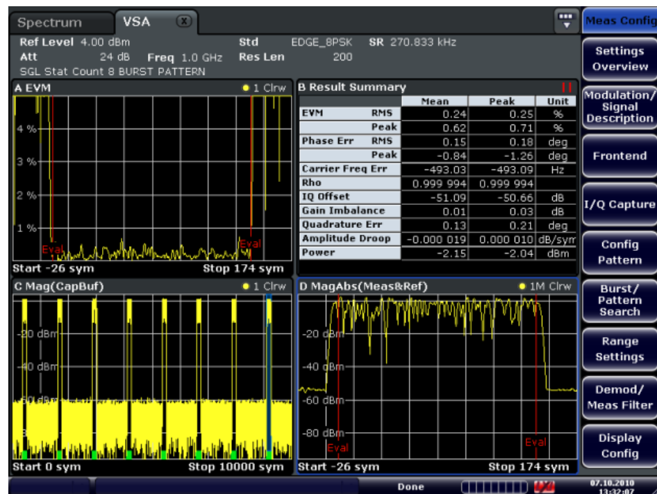
Fig. 9-10: Result range that exceeds the burst length
